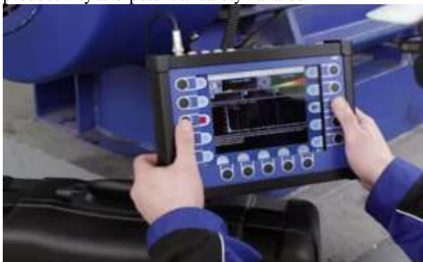
Figure 1. Equipment used in vibration analysis (Source: V-Tech Engineering www.vtechengineer.com/ )
